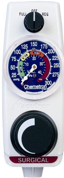
The surgical suction regulator is designed for use in surgical suites. There are two operational modes: regulated vacuum and full line. Regulated suction allows the clinician to set the vacuum level between 0 and 300 mm Hg. On full line mode, the vacuum pressure delivered is unregulated and equal to the vacuum line pressure.
