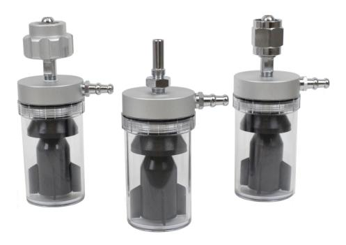
Vacuum traps help safeguard vacuum regulators, wall outlets and the central vacuum system from accidental contamination from canister overflows. This is accomplished by a mechanical float which cuts off suction in the event of a canister overflow.
